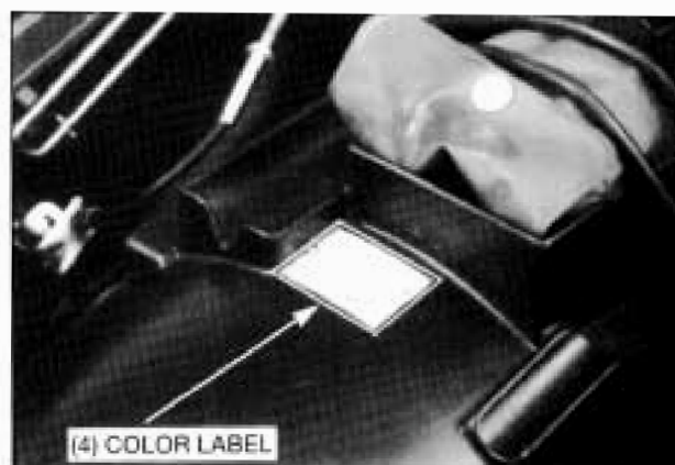
(4) The color label is attached on the rear fender of the under the seat. When ordering color-coded parts, always specify the designated color code.
