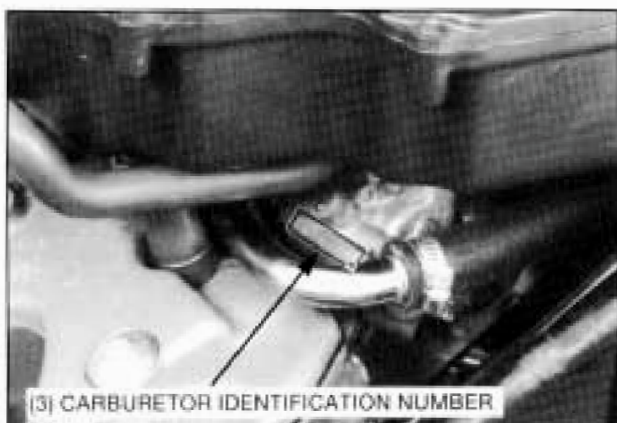
(3) The carburetor identification numbers are stamped on the intake side of the carburetor body as shown.
